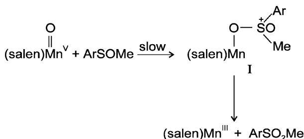
Scheme 1. Mechanism of [(\text{salen})\text{Mn}^{\text{V}}=\text{O}]^+ oxidation of organic sulfoxides.
